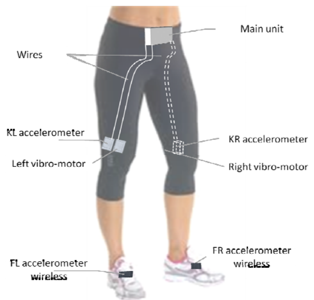
Fig. 1. The wearable running assistant with two rumble devices and four accelerometers mounted on spandex shorts and shoes.
