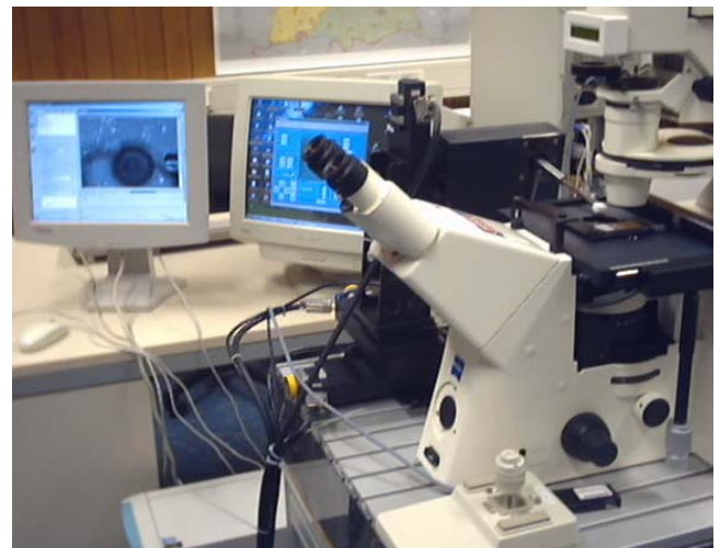
Fig. 19. Experimental set-up for cell penetration (source: F. Ionescu © )
