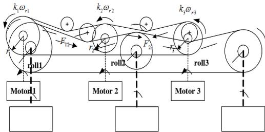
Fig.1. Three-motor synchronous system
