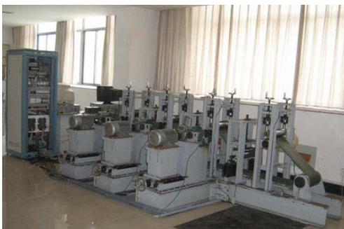
Fig. 8 Experimental platform of three-motor synchronous system
