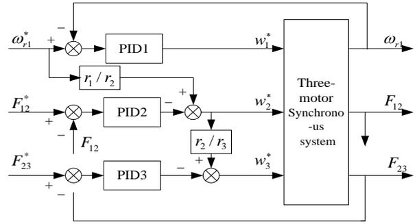
Fig.2 .Structure of PID control system
