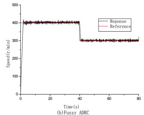
Fig.9 Response of speed tracking square wave
