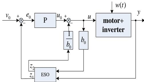
Fig.5 The simplification block diagram of one-order ADRC
