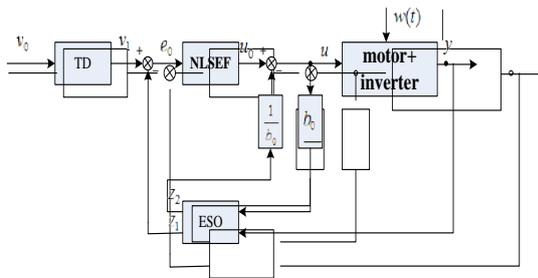
Fig.4 .The block diagram of first-order ADRC
