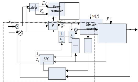
Fig.6 The block diagram of one-order fuzzy ADRC
