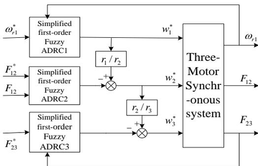
Fig.7 Structure of fuzzy ADRC control system
