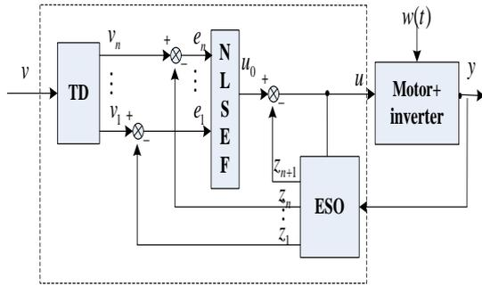
Fig.3. The structure of ADRC
