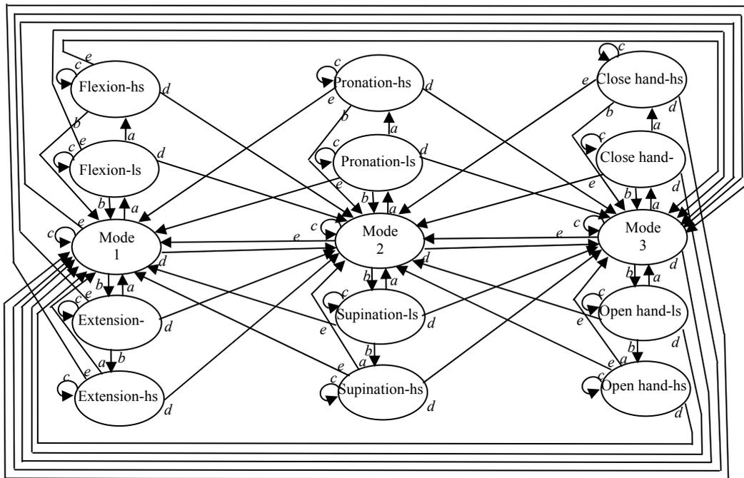
Fig.12 State transition diagram of a finite state machine based controller for an upper-limb prosthesis
