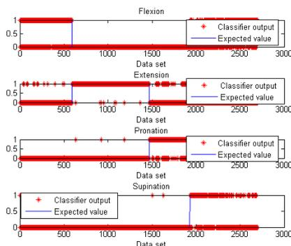
Fig. 11. Comparison between the expected and the obtained results of the classifier when a threshold was used
