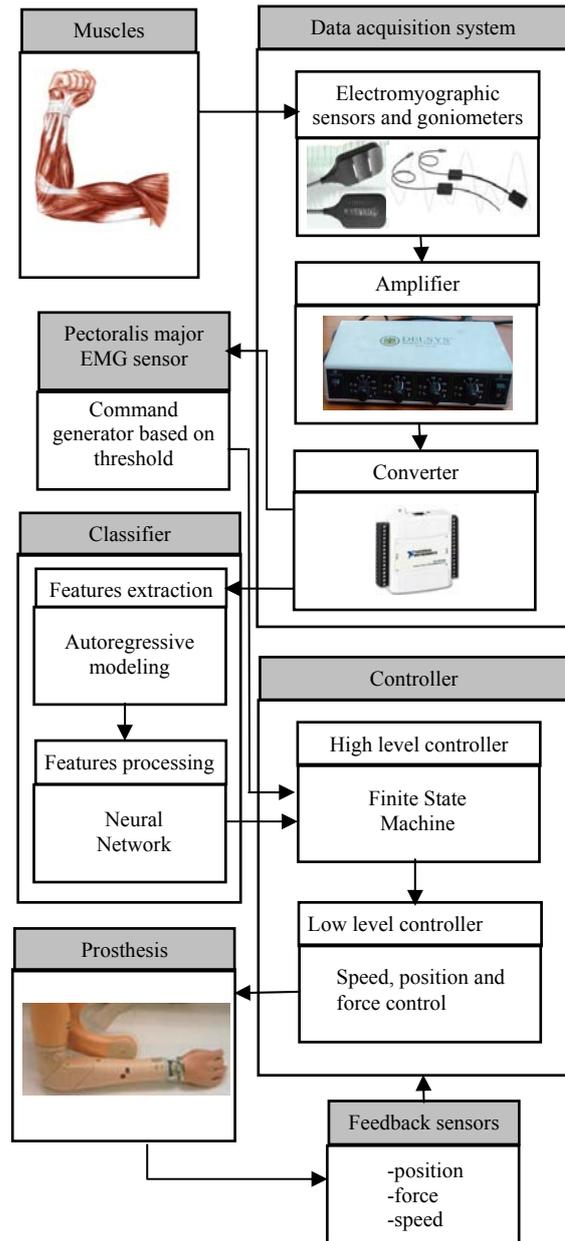
Fig. 2. Myoelectric control system architecture
