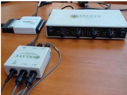
Fig. 3. Bagnoli 4 acquisition system for SEMG signals: -top right: the main amplifier; -bottom left; the input module; -top left: the converter.
