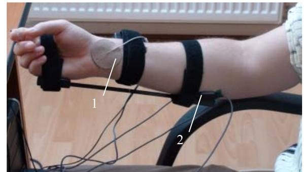
Fig. 6. Position of the sensors (inside view of the forearm): 1- reference electrode , 2- SEMG sensor 2
