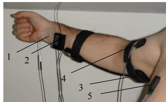
Fig. 7. Position of the sensors on the upper limb: 1-reference electrode, 2-the goniometer for pronation-supination, 3-the goniometer for flexion-extension, 4-SEMG sensor on biceps, 5-SEMG sensor on pectoralis major
