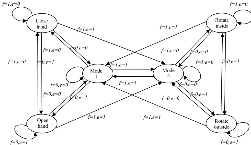
Fig. 10 State transition diagram of finite state machine based controller for hand prosthesis
