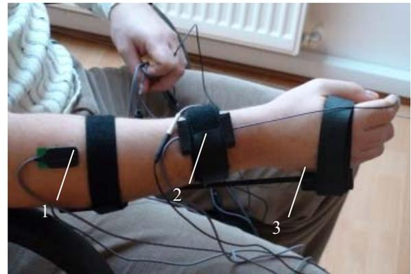
Fig. 5. Position of the sensors (outside view of the forearm): 1- SEMG sensor 1, 2-small goniometer, 3-large goniometer.
