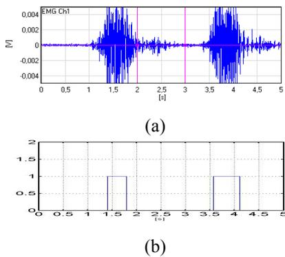
Fig. 1. (a) SEMG signal recorded, (b) Threshold control command generated
