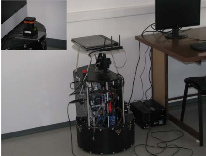
Fig. 1 Laser rangefinder Hokuyo UTM-30LX (detail in left upper corner) mounted on Indoor Mobile Robot.
