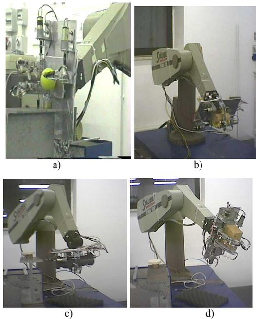
**Fig. 10.** A prototype of LARM Hand 1 attached to the wrist of a robot PUMA 562: a) grasping a tennis ball; b) grasping a cylinder of wood with radius  $r=50$  mm; c) grasping a cylinder of teflon with radius  $r=30$  mm; d) grasping a cube of wood with side  $l=60$  mm.
