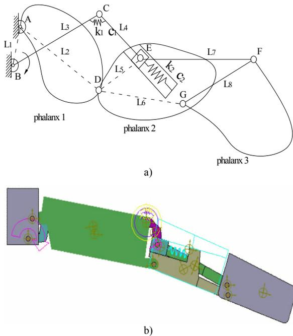
**Fig. 5.** A new 1-DOF LARM finger mechanism for underactuated grasping operation: a) a kinematic scheme; b) a 3D CAD model.
