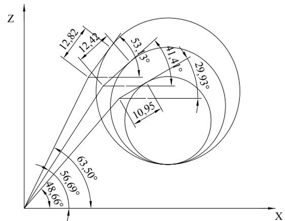
**Fig. 3.** A scheme for grasping cylindrical objects with radius  $R$  from 30 to 50 mm.
