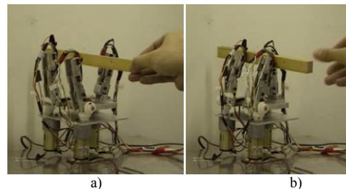
**Fig. 11.** A prototype of LARM Hand 2 while grasping a thin box of wood with side  $l=10$  mm: a) approaching motion; b) firm grasping.
