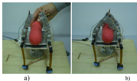
**Fig. 12.** Main phases of a tests carried out by using the position control with force feedback: a) positioning the object on the palm ; b) grasping the object.
