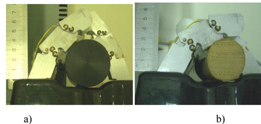
**Fig. 4.** Contact point of a finger of LARM Hand IV with cylindrical objects of different radius  $r$ : a) when  $r=50$  mm; b) when  $r=30$  mm.
