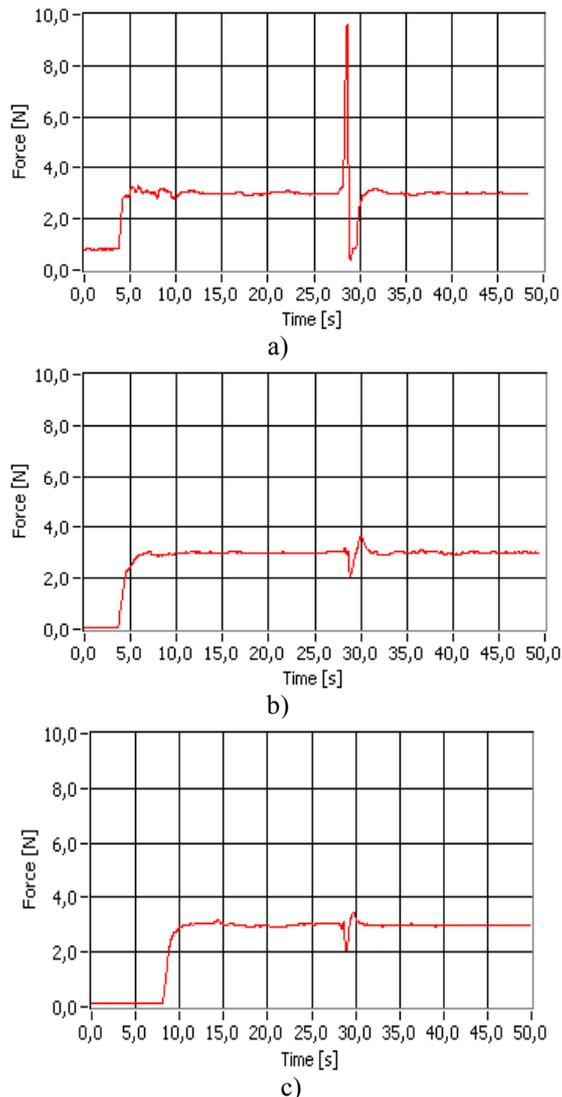
**Fig. 13.** Measured grasping forces during the grasping of a balloon filled with flour in Fig.12 (when the position control with force feedback is used and a random impulsive force is applied on finger 1 at about 28s): d) a) sensor on finger 1; b) sensor on finger 2; c) sensor on finger 3.
