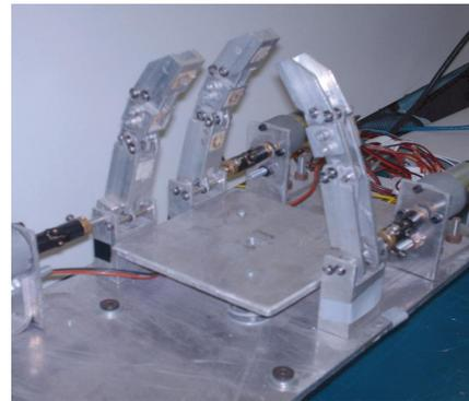
**Fig. 7.** A built prototype of LARM Hand 1 at LARM in Cassino.
