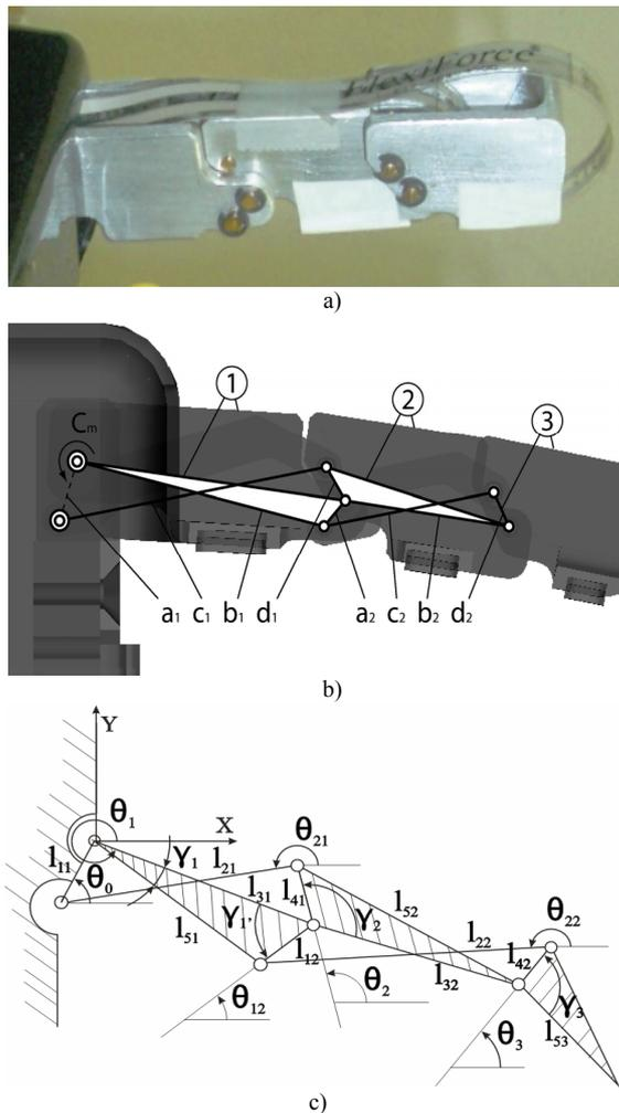
**Fig. 2.** A finger of LARM Hand: a) a preliminar prototype at LARM; b) a 3D CAD model; c) a kinematic model for the driving mechanism .
