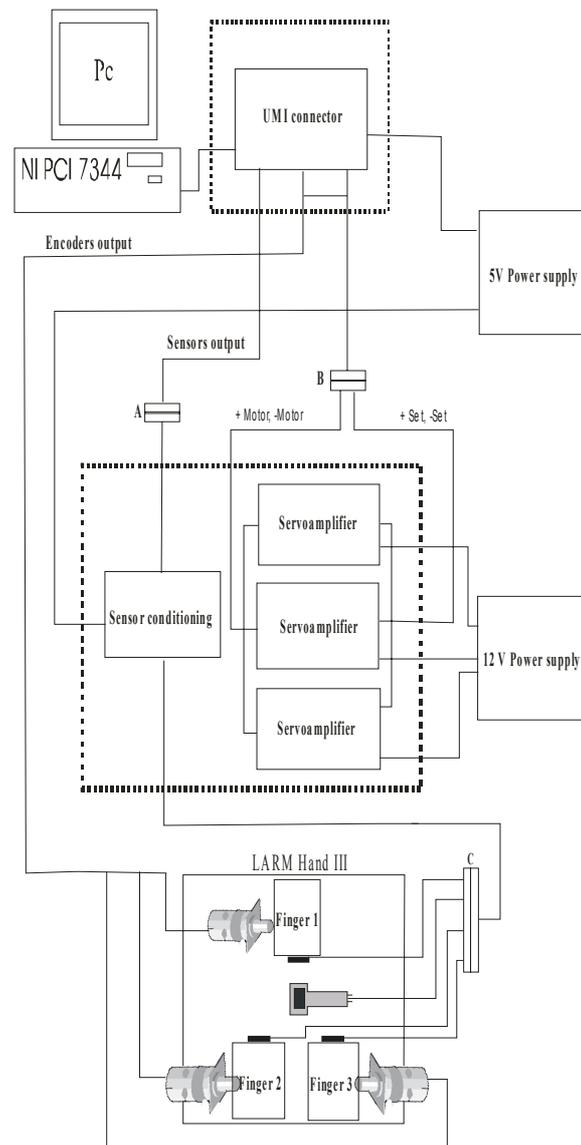
**Fig. 6.** A scheme of the hardware that is needed for the operation of a LARM Hand prototype.
