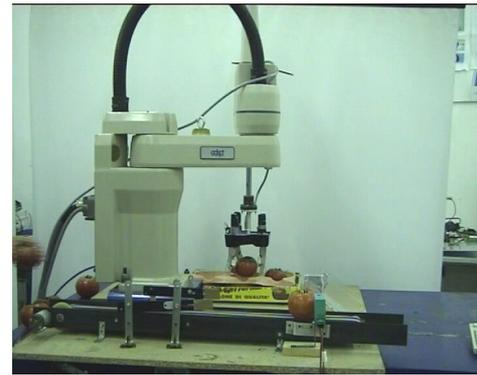
**Fig. 14.** Packaging tomatoes with LARM Hand 4 and a SCARA Adept Cobra robot: a) approaching a tomato on a conveyor belt; b) grasping a tomato; c) handling a tomato.
