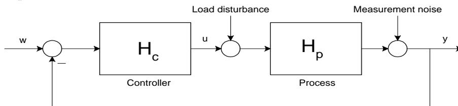
Fig. 1. Control system structure.
