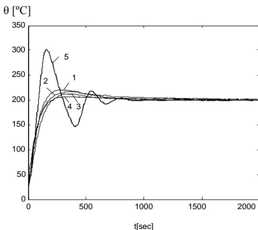
**Fig. 9.** Comparison of the NP1(1), NP2(2), NPS(3), IMC (4), and ZN(5) methods, temperature control of a soldering hammer, step response ( $200^\circ\text{C}$ ).
