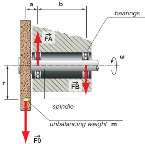
Fig. 2 Grinding wheel and its bearings.
