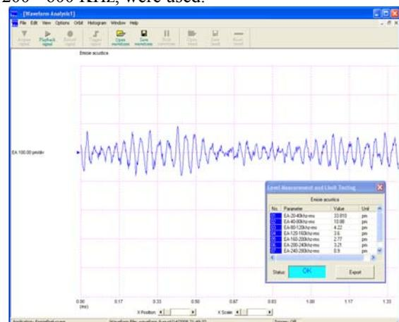
Fig. 6 The waveform of acoustic emissions – new disk processing.
