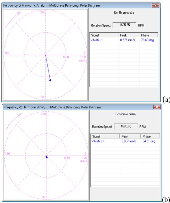
Fig. 5. The polar diagram of initial vibrations (a) and after balancing (b).
