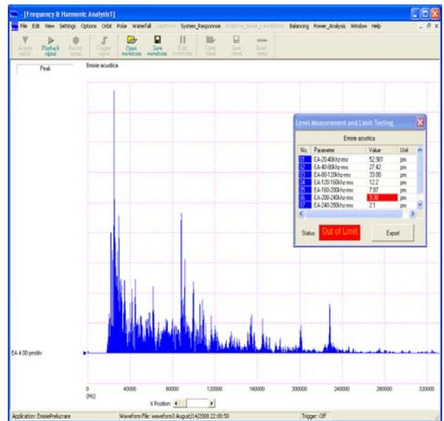
Fig. 9. The frequency spectrum of emissions – with used disk processing.
