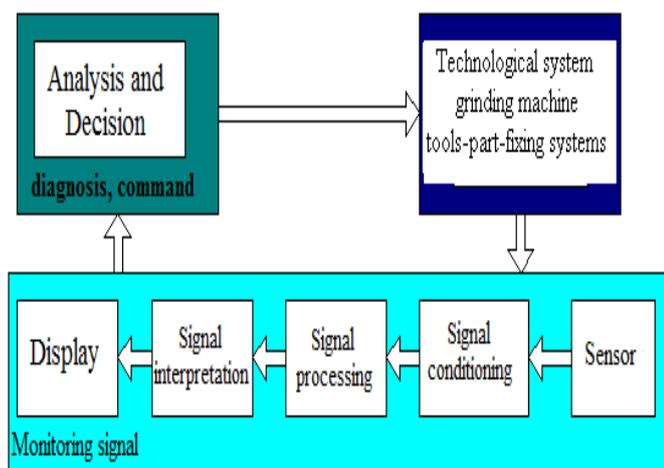
Fig. 10. The control loop of the manufacturing process.
