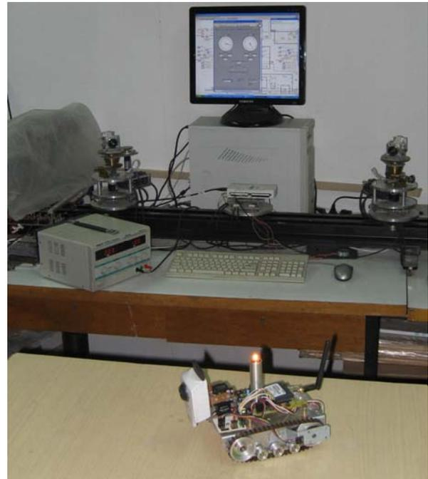
Fig. 3. View of the position tracking installation determining the minirobot's coordinates
