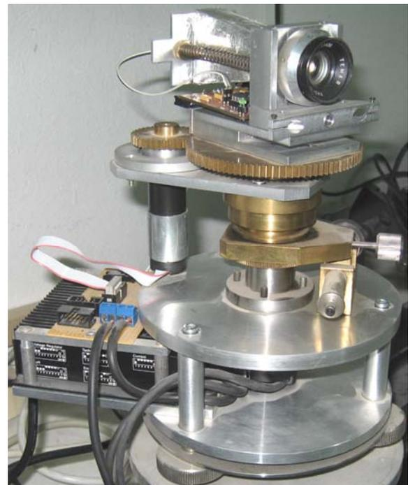
Fig. 4. Module including the rotating transducer platform and the attached optoelectronic device
