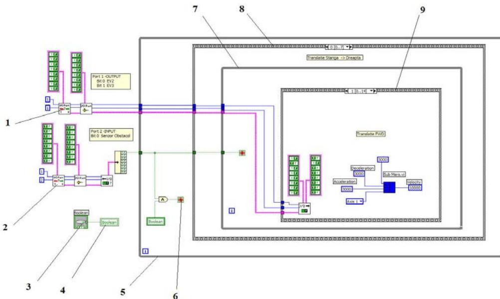
Fig. 15. Block diagram of main control program of the robot.
