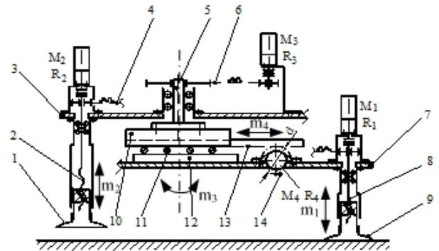
Fig. 2. Cinematic scheme of robot.
