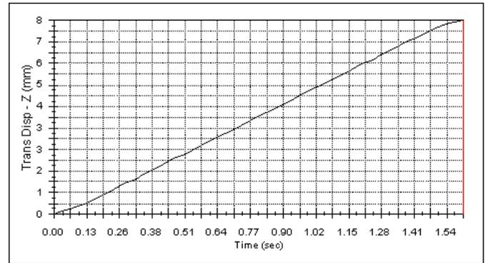
Fig. 10. Displacement variation during the robot translation relative to the cups.
