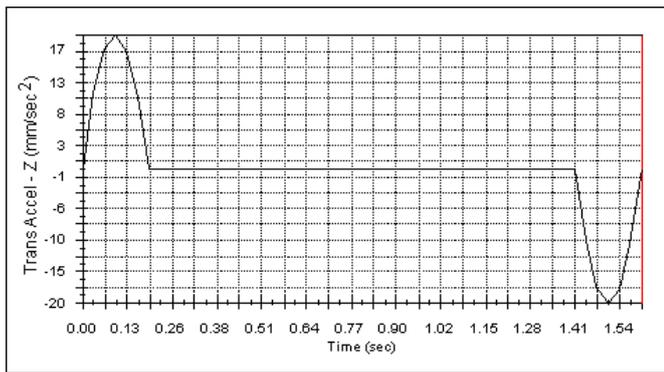
Fig. 8. Acceleration variation during the robot translation relative to the cups.
