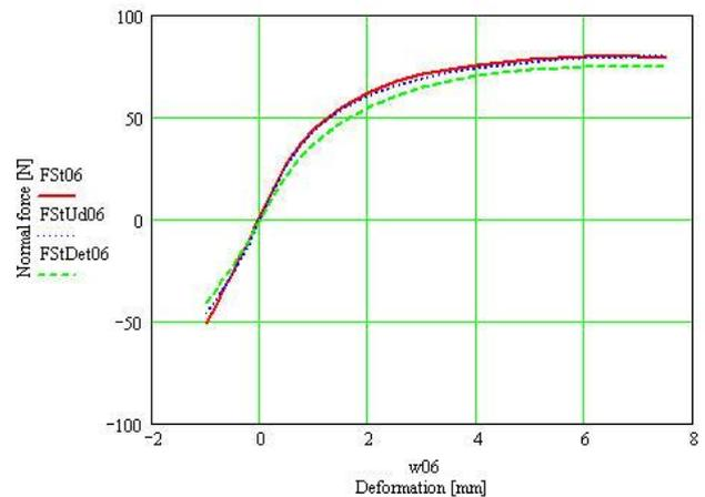
Fig. 6. Cup behaviour on glass for different conditions: *FSt06* – dry surface, *FstUd06* – wet surface with water, *FstDet* – wet surface with detergent for window washing.
