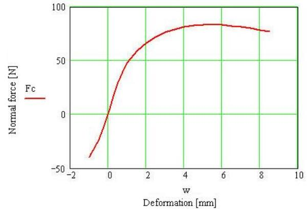
Fig. 5. Cup characteristic for  $\Delta p = 0.57$  bar.
