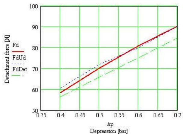
Fig. 7. Cup detachment force from glass for different conditions: *Fd* – dry surface, *FdUd* – wet surface with water, *FdDet* – wet surface with detergent for window washing.
