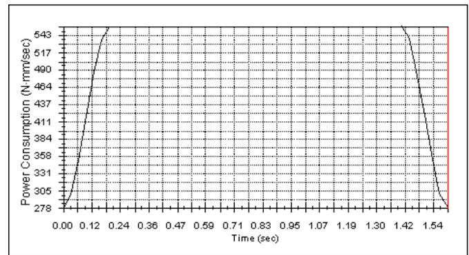
Fig. 11. Instantaneous power variation during the robot translation relative to the cups.
