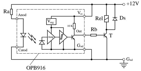
Fig. 12. Scheme of photoelectric circuit.
