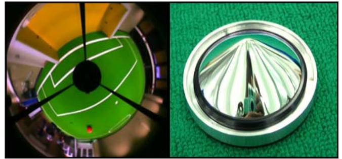
Fig 3. hyperbolic mirror and the typical panoramic image captured.
