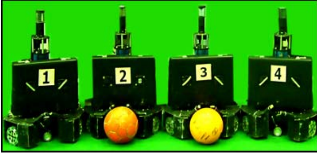
Fig. 1 3-wheeled omni-directional mobile robot with an omni-directional vision system, a normal camera and a kicking device, and is controlled by a notebook PC.
