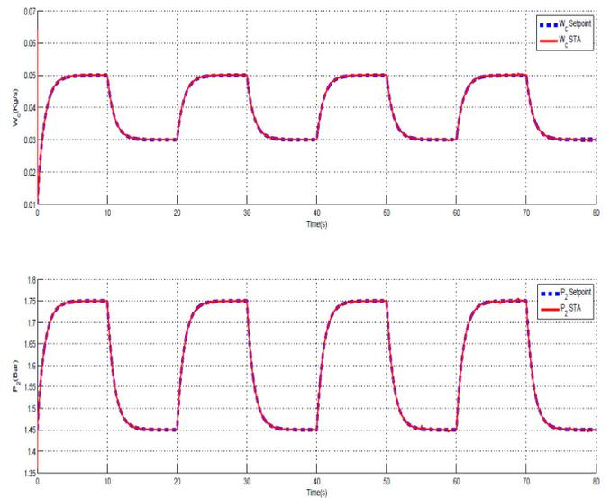
Fig. 6.  $W_c$  and  $P_2$  tracking performance for the STA with Additive leakage time varying faults and multiplicative loss-of-effectiveness time varying faults in  $EGR$  and  $VGT$  actuators [improved gains].
