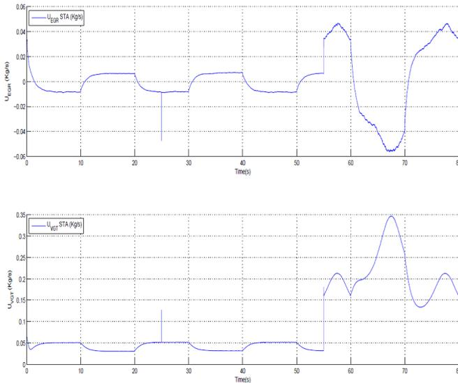
Fig. 7. Control inputs  $U_{EGR}$  and  $U_{VGT}$  for the STA with Additive leakage time varying faults and multiplicative loss-of-effectiveness time varying faults in EGR and VGT actuators [improved gains].
