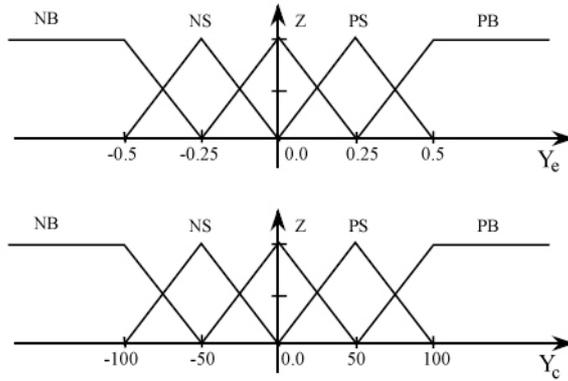
Fig. 5. Membership functions for the input variables of the fuzzy inverse model.
