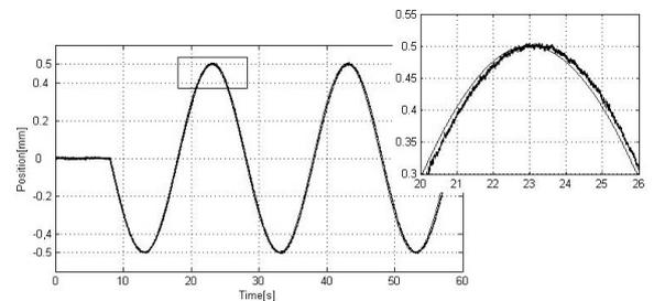
**Fig. 11.** The tracking of a sine trajectory ( $g_p = 1/300$ )
