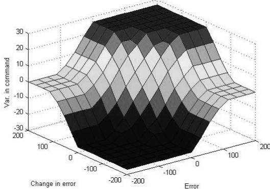
**Fig. 12.** Control surface of the initial Fuzzy-PD system
