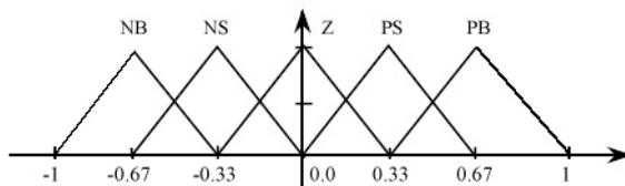
Fig. 6. Normalized domain and membership functions for the output variable of the fuzzy inverse model
