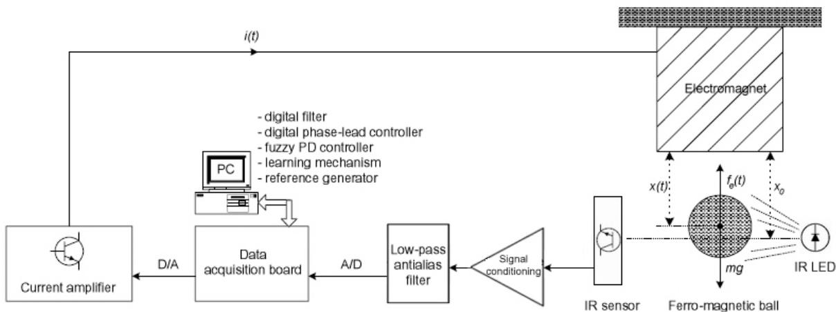
Fig. 7. The implementation of the positioning system based on magnetic levitation controlled by a Learning Fuzzy-PD controller
