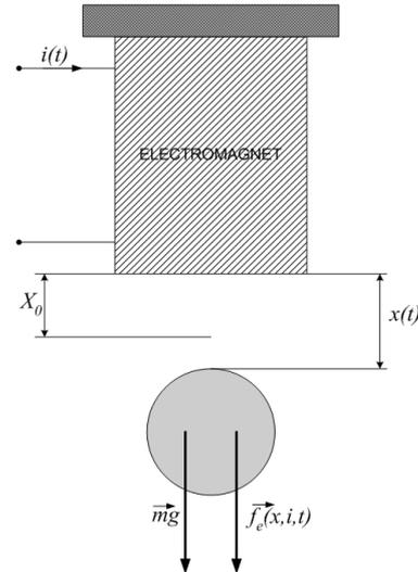
Fig. 1. Electromagnetic levitation
