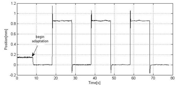
**Fig. 10.** The tracking of a square trajectory
