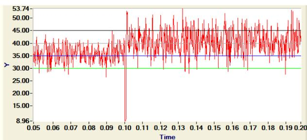
Fig. 18. Indirect adaptive control solution for a  $6.25\%U_0$  SPAB signal amplitude.
