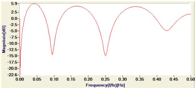
Fig. 9. Frequency representation of the output sensitivity function  $S_{yp}(e^{-j\omega})$ .
