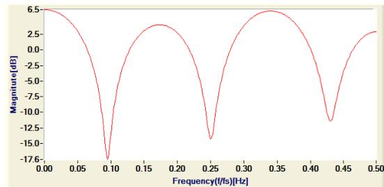
Fig. 6. Frequency representation of the output sensitivity function  $S_{yp}(e^{-j\omega})$ .
