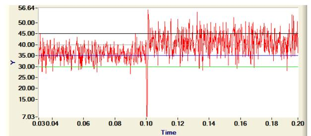
Fig. 13. Indirect adaptive control solution for a  $6.25\%U_0$  SPAB signal amplitude.
