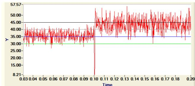
Fig. 11. Indirect adaptive control solution for a  $2.5\%U_0$  SPAB signal amplitude.
