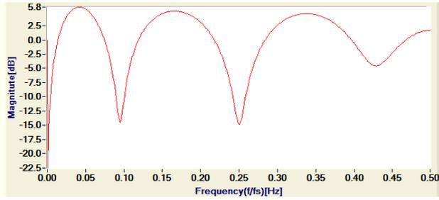
Fig. 8. Frequency representation of the output sensitivity function  $S_{yp}(e^{-j\omega})$ .
