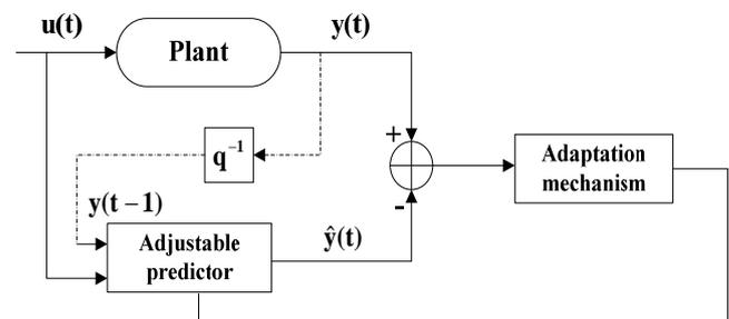
Fig. 1. Indirect adaptive control scheme.
