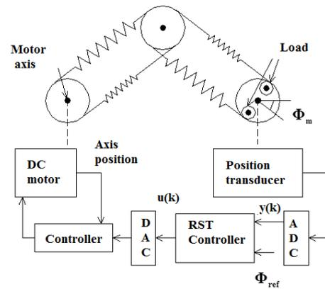
Fig. 2. Control scheme of the flexible transmission system.
