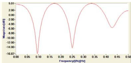
Fig. 3. Frequency representation of the output sensitivity function  $S_{yp}(e^{-j\omega})$ .
