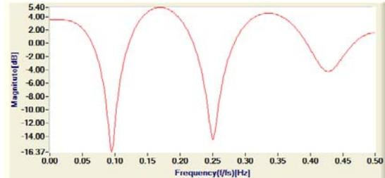
Fig. 5. Frequency representation of the output sensitivity function  $S_{yp}(e^{-j\omega})$ .
