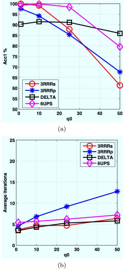
Figure 8. Performance evaluation results. (a): percentage of convergence for an accuracy given by Acc1.(b): average of iteration needed to find an accurate solution.
