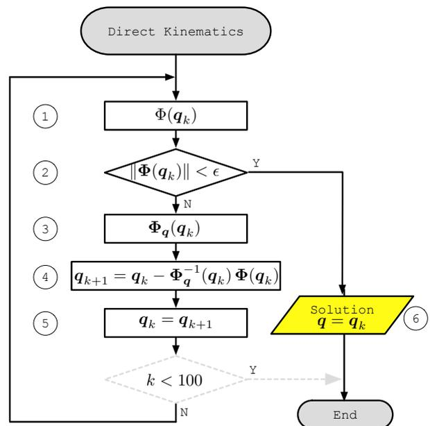
Figure 1. Direct Kinematics Algorithm.
