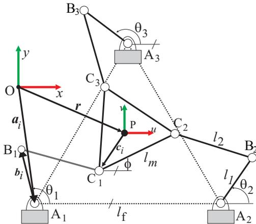
Figure 3. Schematic diagram of the Planar-3RRR PM.
