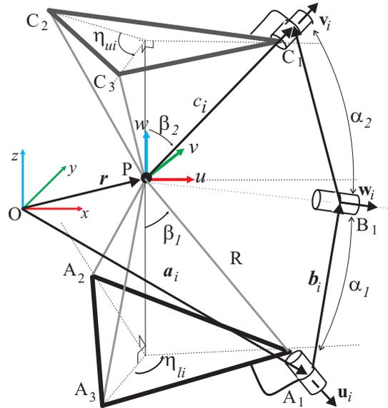
Figure 4. Schematic diagram of the Spheric-3RRR PM.
