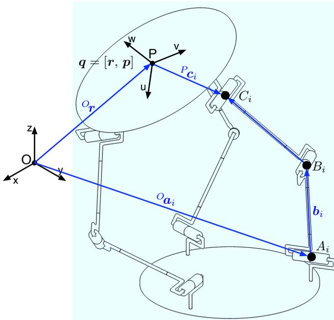
Figure 2. Schematic diagram of a two-links leg of a generic PM.
