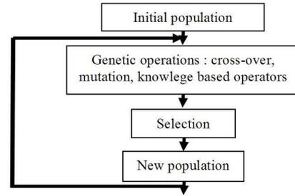
Fig. 9. Flow chart of a genetic algorithm
