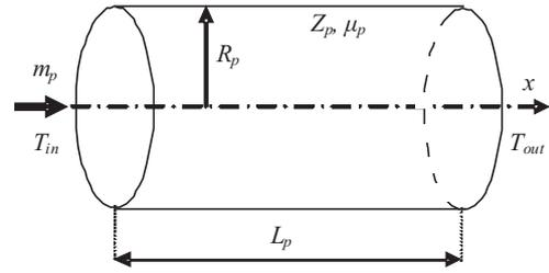
Fig. 2. Notations for pipes modeling
