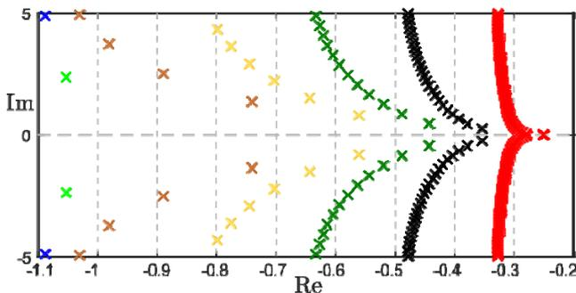
Fig. 4. Roots locus of (4) when  $\sigma$  is fixed and  $k_i$  is varied.  $\hat{k}_i = \{(x) 0.5, (x) 0.66, (x) 0.82, (x) 0.97, (x) 1.1, (x) 1.3, (x) 1.5\}$
