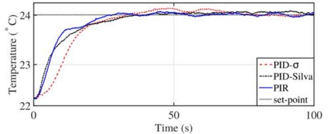
Fig. 8. Real system response of QNET-HVACT.
