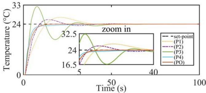
Fig. 3a. System response (1)-(2) when  $\sigma$ ,  $k_p$  and  $k_i$  are fixed and  $k_r$ ,  $h$  are varied.
