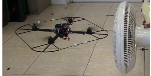
Fig. 23. Hummingbird quadrotor under perturbations.
