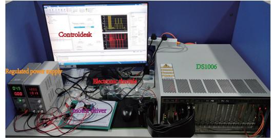
Fig. 3. HIL test platform of electronic throttle system.
