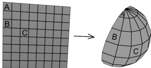
**Fig. 1.** Correspondence between a square surface and a half of sphere
