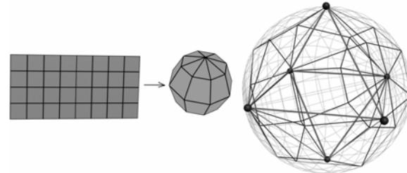
**Fig. 3.** Iteration 2: Subdivision of the sphere into 32 sides
