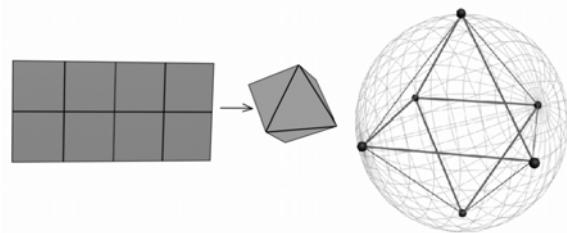
**Fig. 2.** Iteration 1: Subdivision of the sphere into 8 sides
