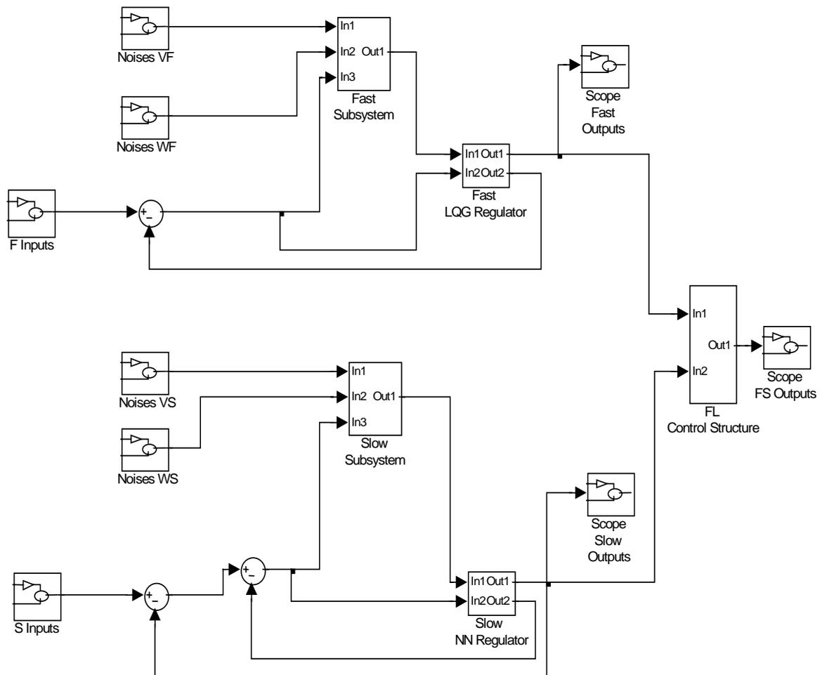
**Fig. 1.** The block scheme of a two-rate decentralized control system.
