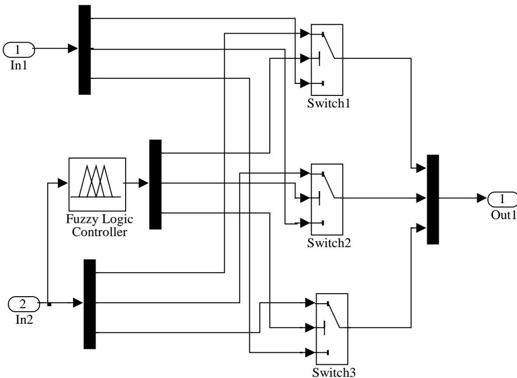
Fig. 4. The block scheme of the FL control structure.
