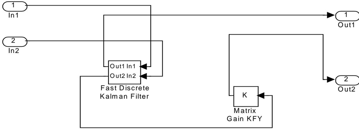
Fig. 2. The block scheme of the fast LQG regulator.
