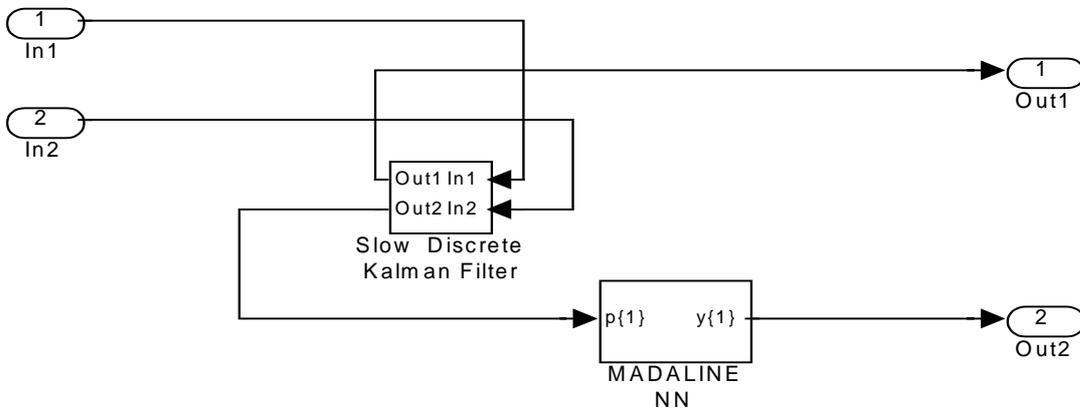
Fig. 3. The block scheme of the slow NN regulator.
