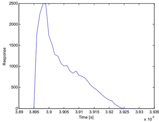
Fig. 2. Spatial impulse responses from 2D linear array with 20 elements
