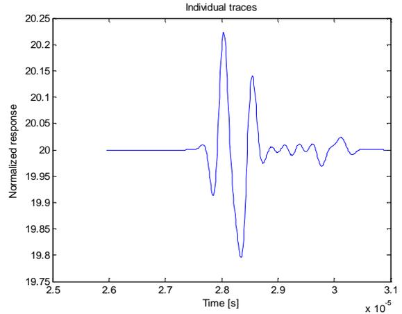
Fig. 4. The individual trace from 20<sup>th</sup> element of linear array
