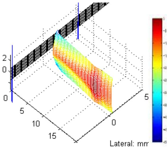
Fig. 5. Ultrasound beam profile simulation for linear array with 64 elements (by courtesy BioSono Inc.)
