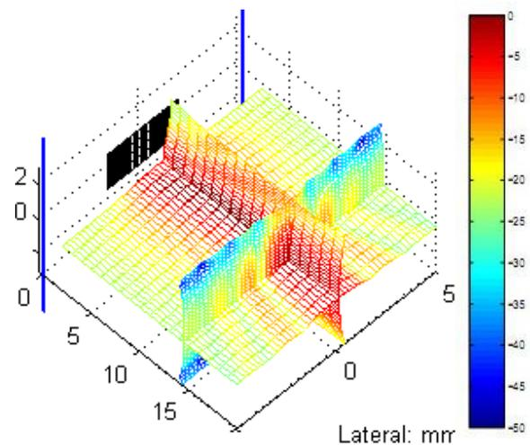
Fig. 6. Ultrasound beam profile simulation for linear array with 20 elements, in X-Y&Y-Z&X-Z planes (by courtesy BioSono Inc.).
