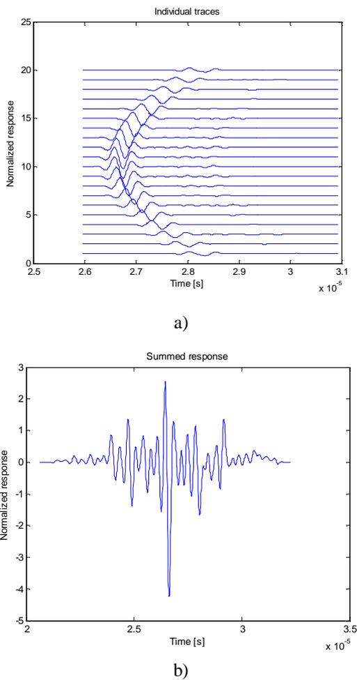
Fig. 3. (a) The individual responses and (b) the summed response, from 20 element linear array
