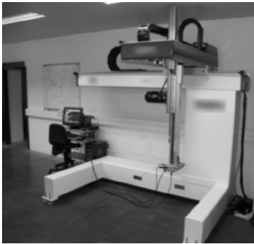
Fig. 6 Overview of the test-setup prototype (maximum feedrate: 120 m.min -1 , maximum acceleration: 4 m.s -2 ).
