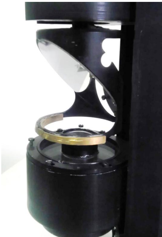
Fig. 22 Spinning mirror assembly manufactured prototype
