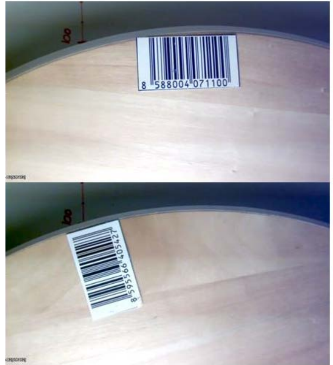
Fig. 12: Rolling shutter effect - static image
