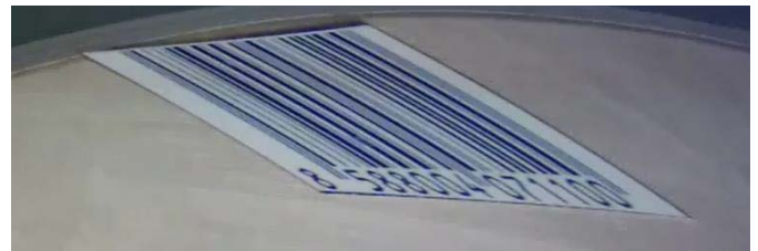
Fig. 13: Image blur due to the motion (3 m/s code movement speed)
