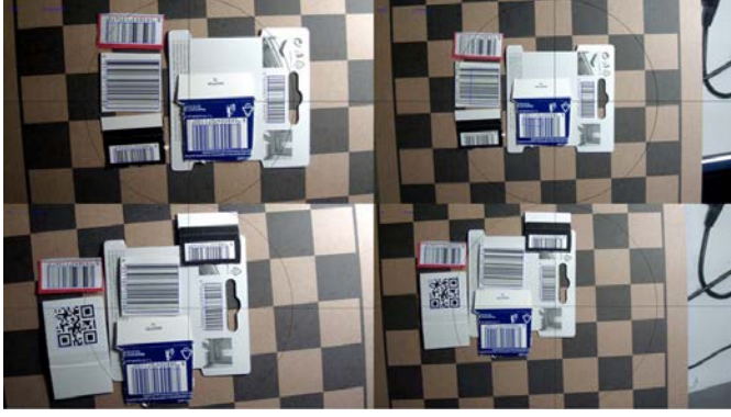
Fig. 4: Scanned scene used in the measurement of success of the code detection: top left - Measurement 1 [1280x720 pixels; 35 cm] top right - Measurement 2 [1280x720 pixels; 46 cm] bottom left - Measurement 3 [1920x1080 pixels; 35 cm] bottom right - Measurement 4 [1920x1080 pixels; 46 cm ])
