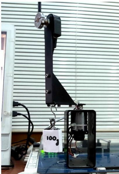
Fig. 9. Pendulum setup with 0.10 kg mass attached to arm
