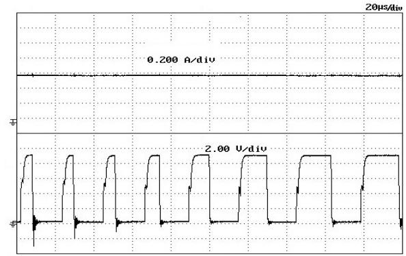
Fig. 6 PWM rectangular wave for unstable closed loop
