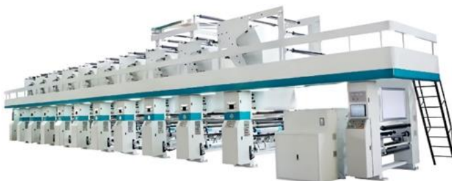
Fig. 1. A R2R printing system used in the industry. Note. R2R: Roll-to-roll.
