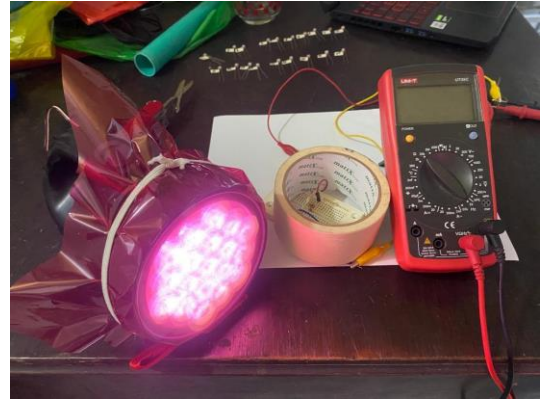
Figure 4. LDR under the influence of a filtered light stimulus
