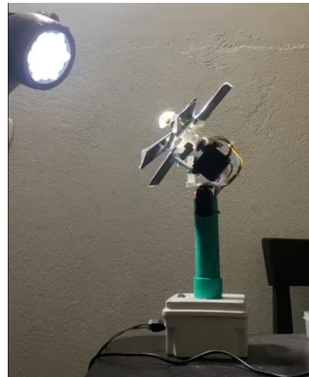
Figure 20. Scale prototype following light from a flashlight.
