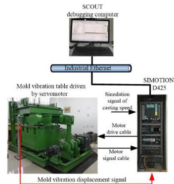
Fig. 8. Servo motor control cabinet and vibration platform of continuous casting mold.
