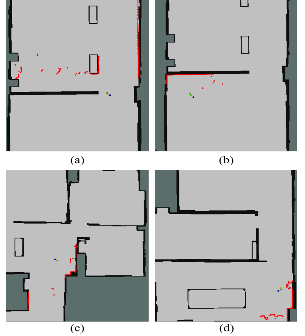
Fig. 9. Comparison of localization results for Ubot at test locations. The actual positions (green points), estimated positions from the EKF-based method (yellow points), and estimated positions from the IAMCL-based method (blue points) are shown at Locations (a) A, (b) B, (c) C, and (d) D.
