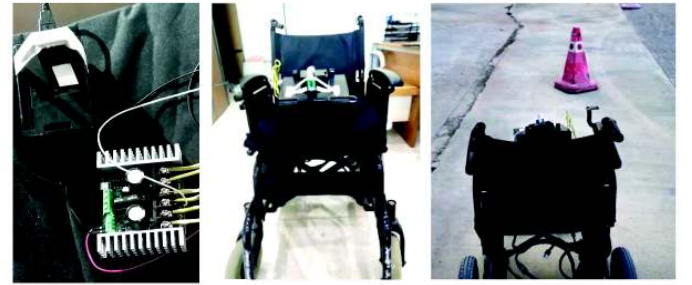
Fig. 8. The PWC used during experiments and development with the installed hardware (battery, Raspberry Pi, motor controller, and camera).
