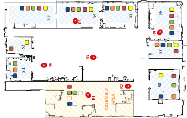
Fig. 6. Simulation snapshot of the transportation scenario with six Pioneer P3DX robots at time t = t' .
